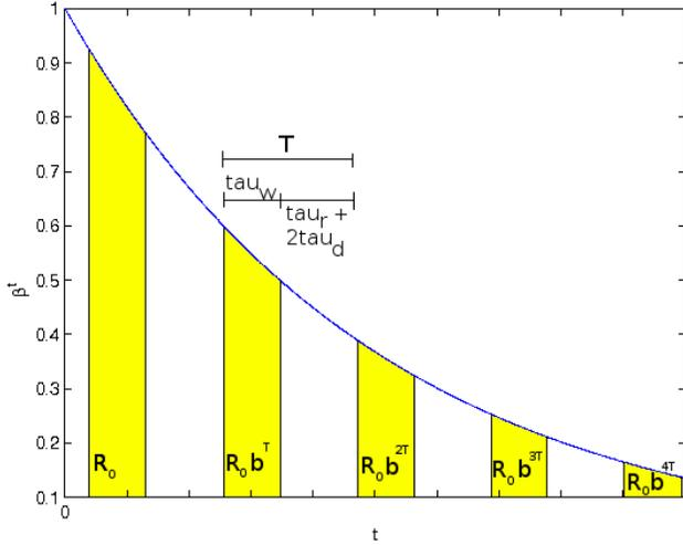
Figure 2: General discounting in refuel - work cycles. The shaded areas are periods in which the robot works and thus earns a reward. The white areas correspond with time in which the robot does not obtain any rewards because it either travels or refuels
