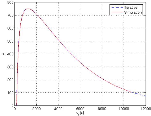
Figure 5: Comparing analytical and simulation results for accumulated reward from a **cyclic** task depending on refuelling time with an example configuration  $I_c = 2.0, I_d = 2.0, I_w = 4.0, \beta = 0.9997, \tau_d \approx 85$
