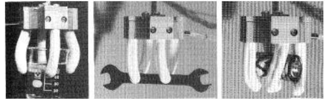
Figure 10: Flexible Microactuator [14]
