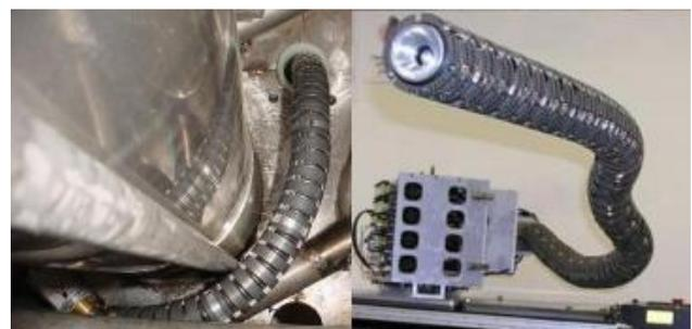
Figure 7: Real Snake-Arm Robots from OC Robotics [28]
